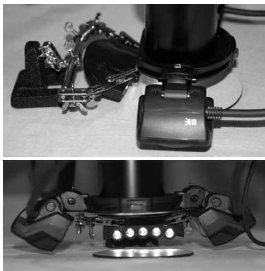
Figure 3. Electrical 'crabs' arms' stand holding LED focussing light. Top: Side view. Bottom: Front view.
